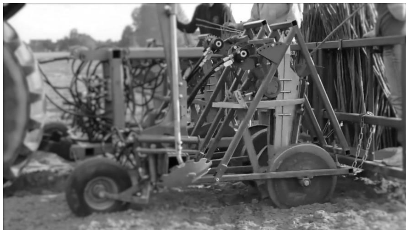
Fig. 13. Three-row plant setter of energy willow rods Step planter 3-reihig - Ernte Stemster. Source: Lignovis
