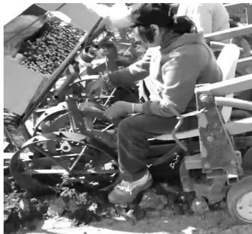
Fig. 7. Plant setters with the radial planting unit with grabs. Source: BioneraVideos (screenshot from the movie)
