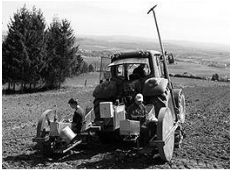
Fig. 9. Energy willow plant setter with a disk planting machine. Source: www.probstdorfer.at
