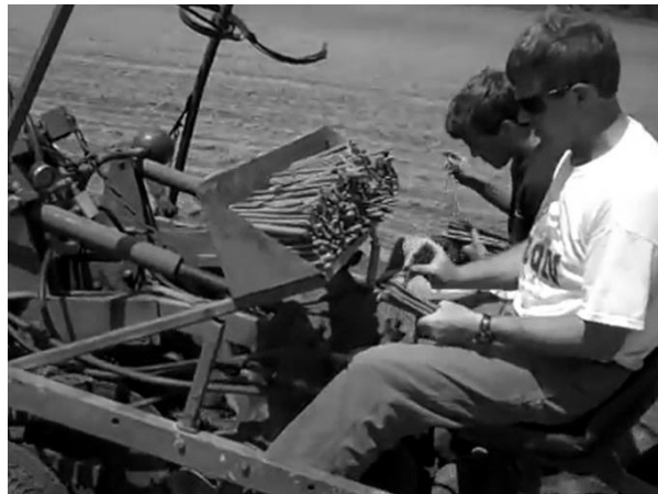
Fig. 5. Energy willow plant setter with manual feeding of cuttings. Source: Willowpedia
