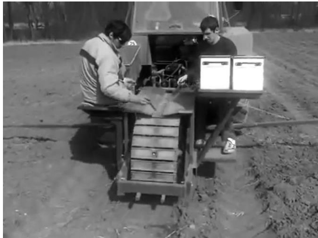
Fig.14. The plant setter of energy willow with a planting unit that look like a caterpillar wimatec MATTES GmbH (Germany). Source: http://www.wimatec-mattes.de
