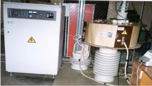
Fig. 7. 20 kW, 1 kHz resonant electric power transmission system.
