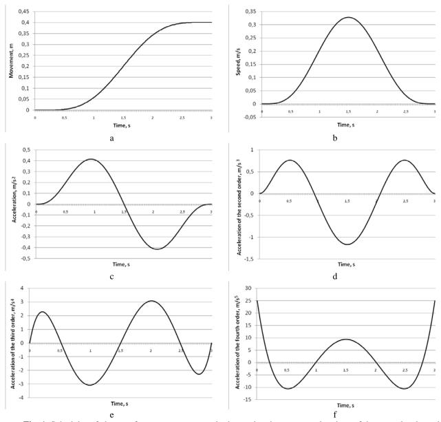
Fig. 1. Schedules of change of movement -a, speed -b, acceleration -c, accelerations of the second order -d, accelerations of the third order -e and accelerations of the fourth order -f at the optimum mode of the movement carts on acceleration of the fourth order.
