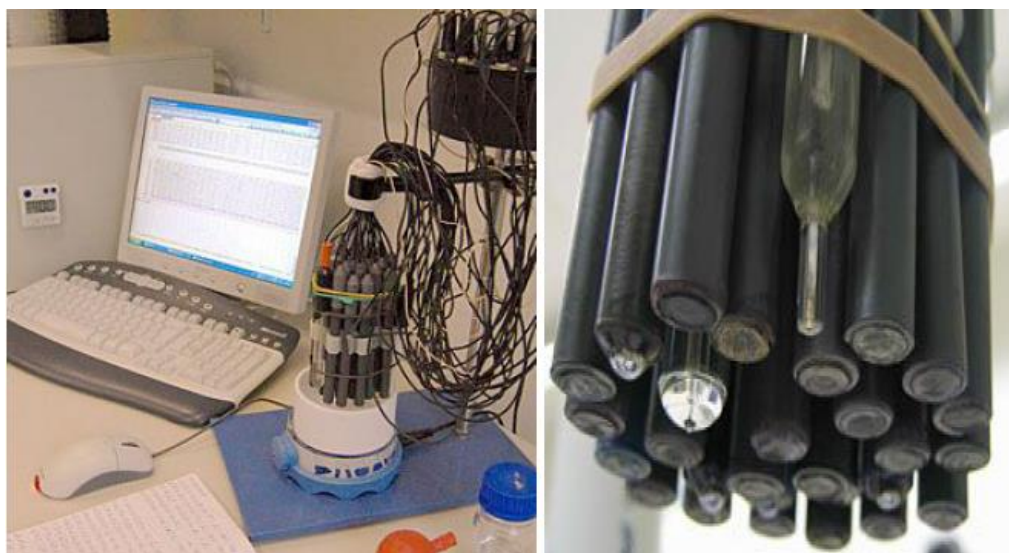
Fig. 1.29. Device "Electronic Tongue"
