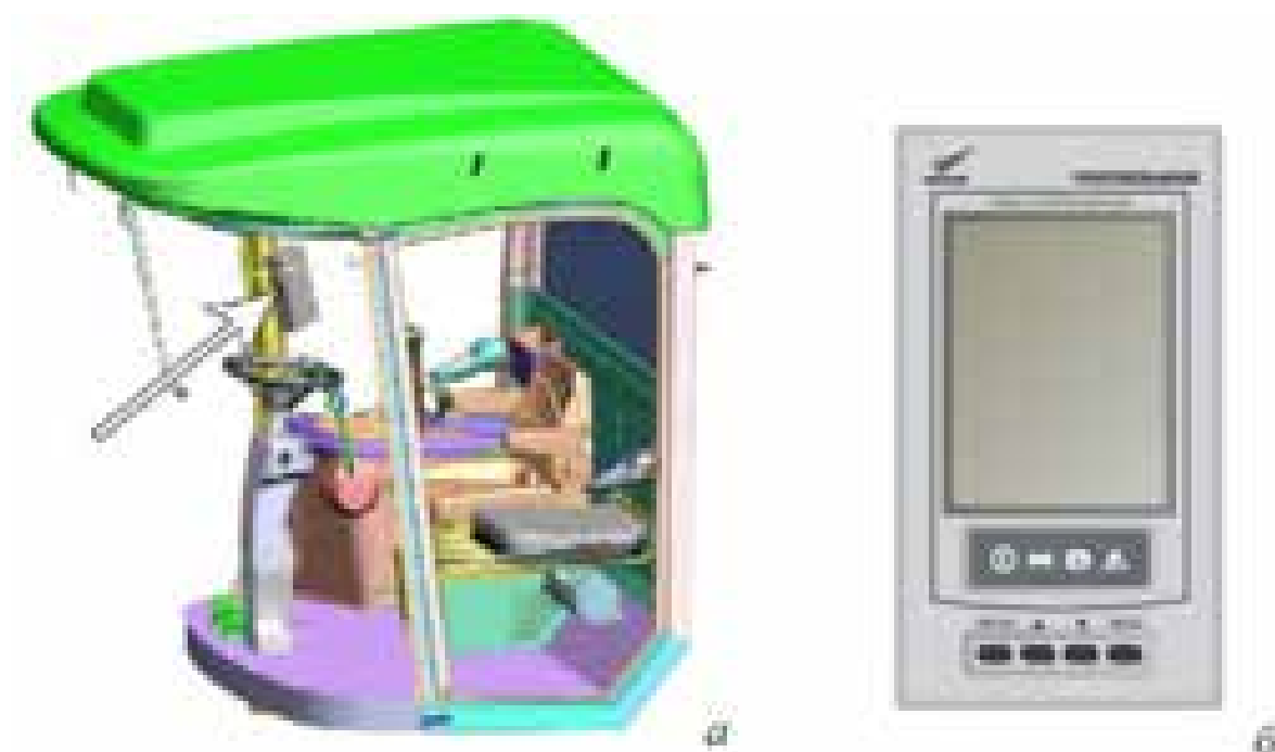
Fig. 3. Information panel PI-142: a – location of the panel; b – appearance of the panel
