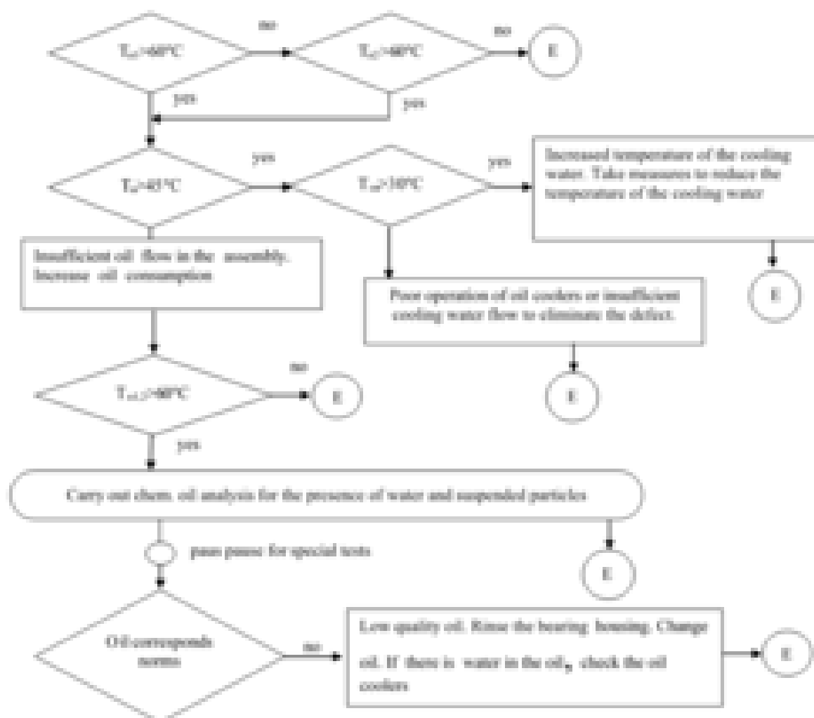
Fig. 1. Fragment of the diagnostic algorithm.
