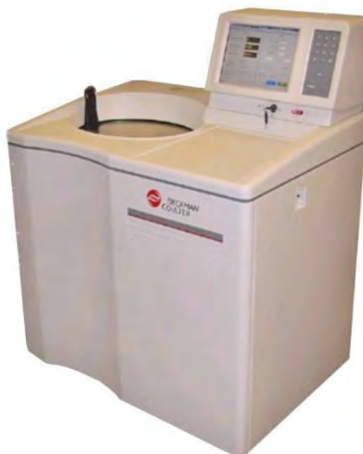
Ultra-centrifuge with ultra-speed, refrigeration, and vacuum system
