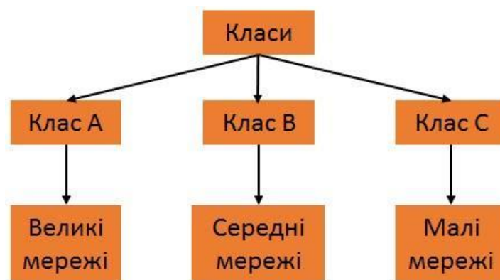
Figure 2.51 - Assignment of classes of IP addresses
