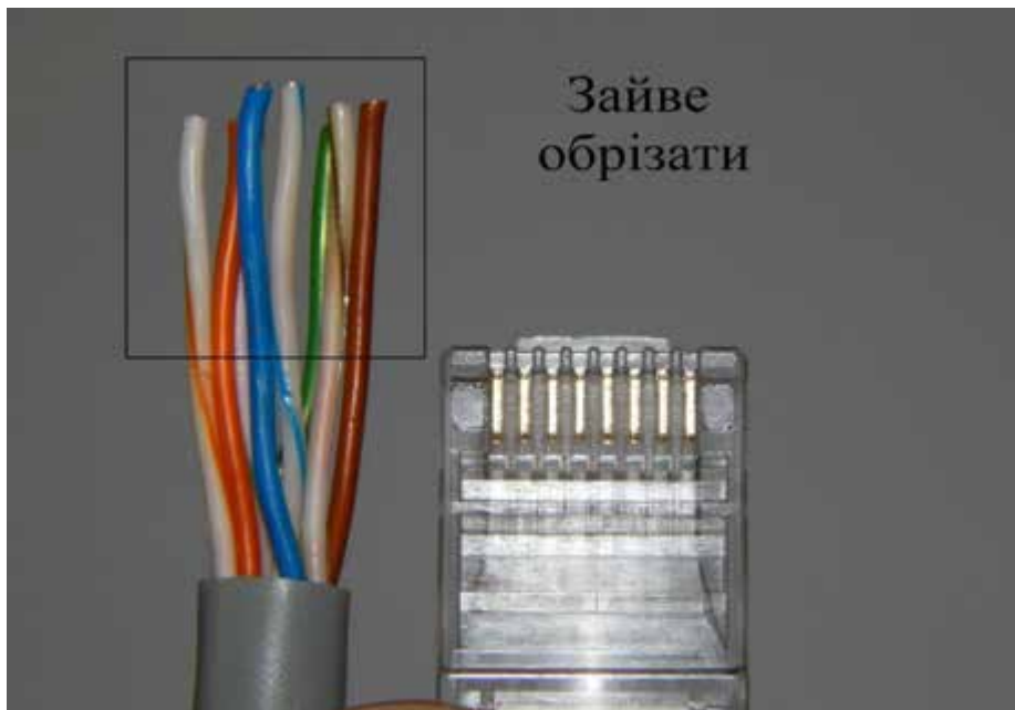
Figure 2.27 – Cutting length of twisted pair wires
