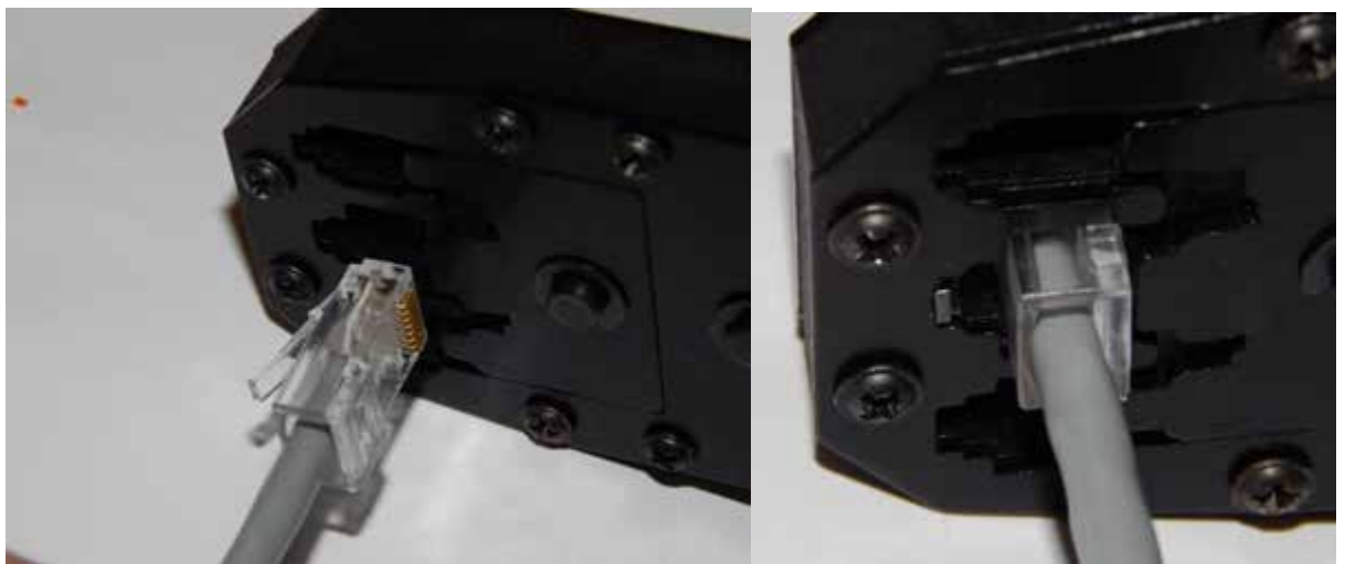
Figure 2.29 – Crimping a connector with an installed pair
