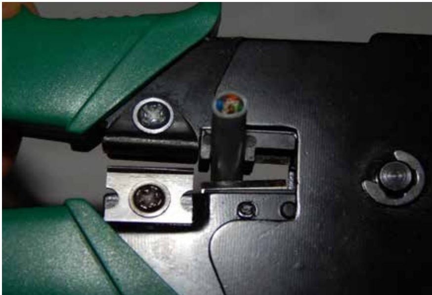
Figure 2.24 – Twisted pair insulation stripping
