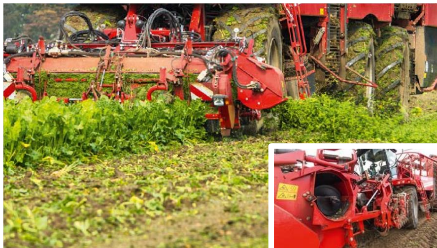
Fig. 1. The combined weed remover provides trouble-free cleaning even with heavy weed growth.
