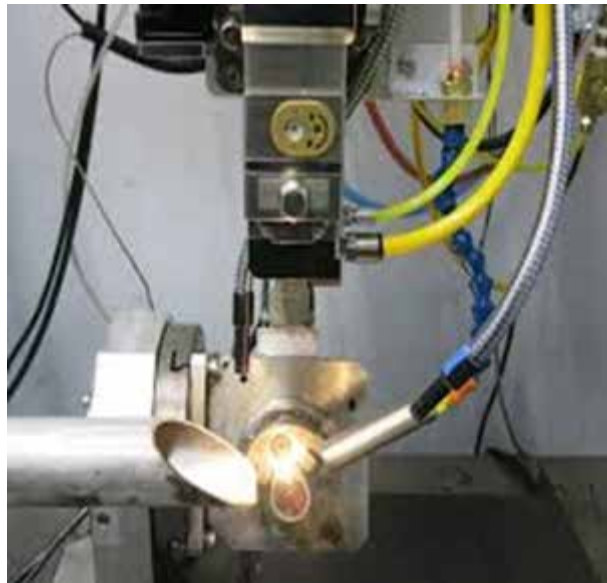
Fig. 1. Electron-beam welding installation
