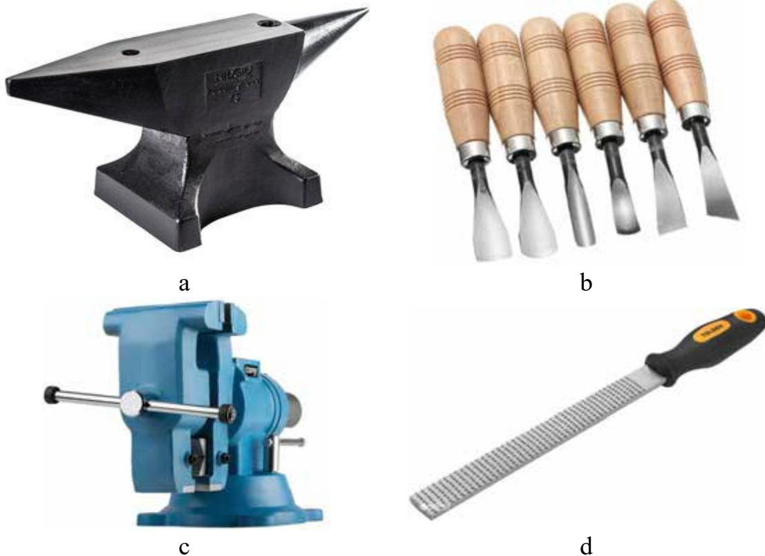
Fig. 2. Application of carbon tool steels: a- anvils; b- chisels; c- vice; d- file.
