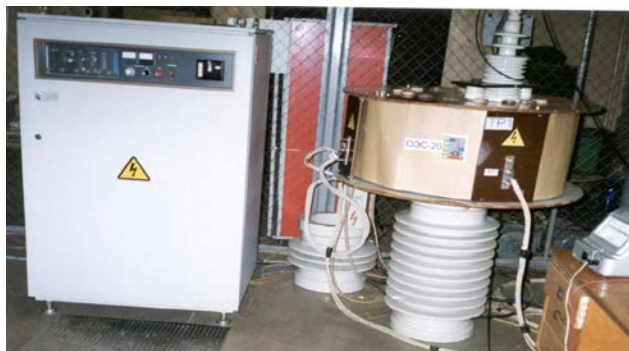
Fig. 7. 20 kW, 1 kHz resonant electric power transmission system.
