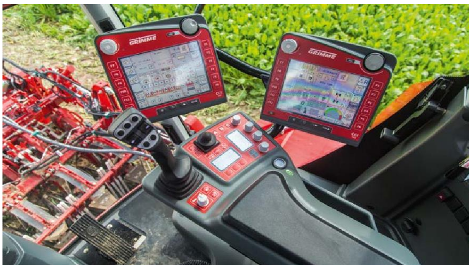
Fig. 2. Ergonomic armrest with programmable elements and control panel.
